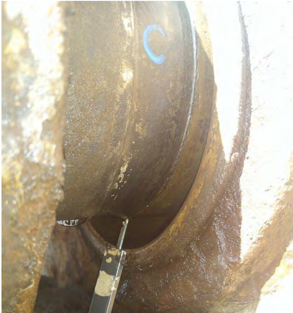
Effect of Clogged Grease Channel
