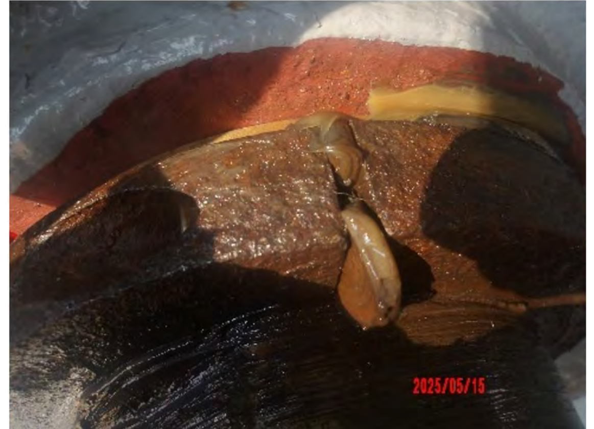
After greasing of the outer Hawser drum bush
