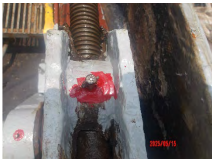
15 May – Before greasing: brake spindle greasing point
