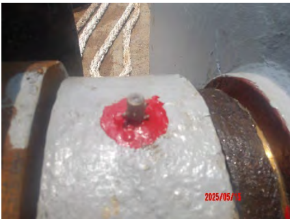
15 May- Before greasing: bushing for side frame outer
