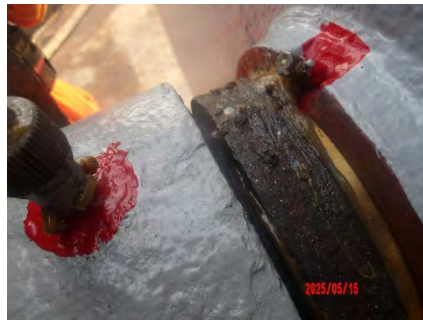
15 May- during greasing: bushing for side frame outer
