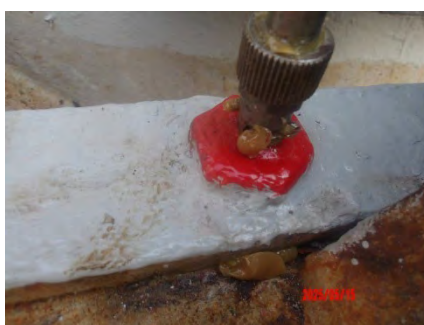
15 May – during greasing: Clutch handle point
