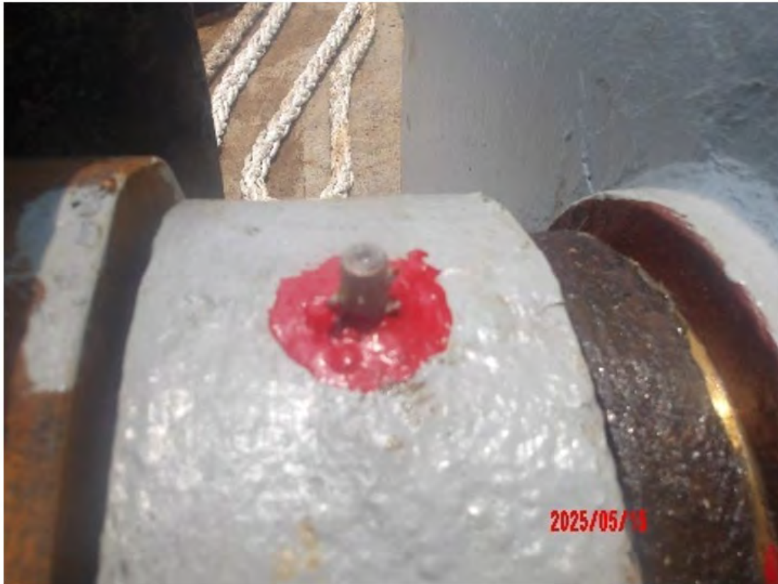
Before greasing of the Outer Side Frame
