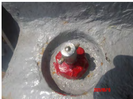
15 May- Before greasing: Clutch of hawser drum 1
