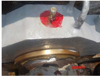
15 May- During greasing : Pinion bush
