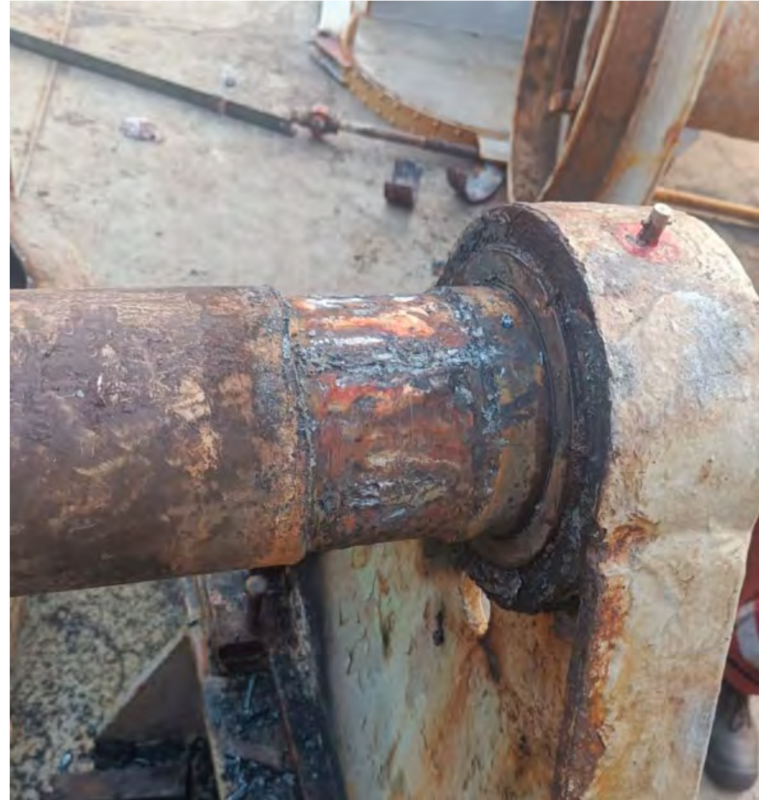
Effect of Clogged Grease Channel
