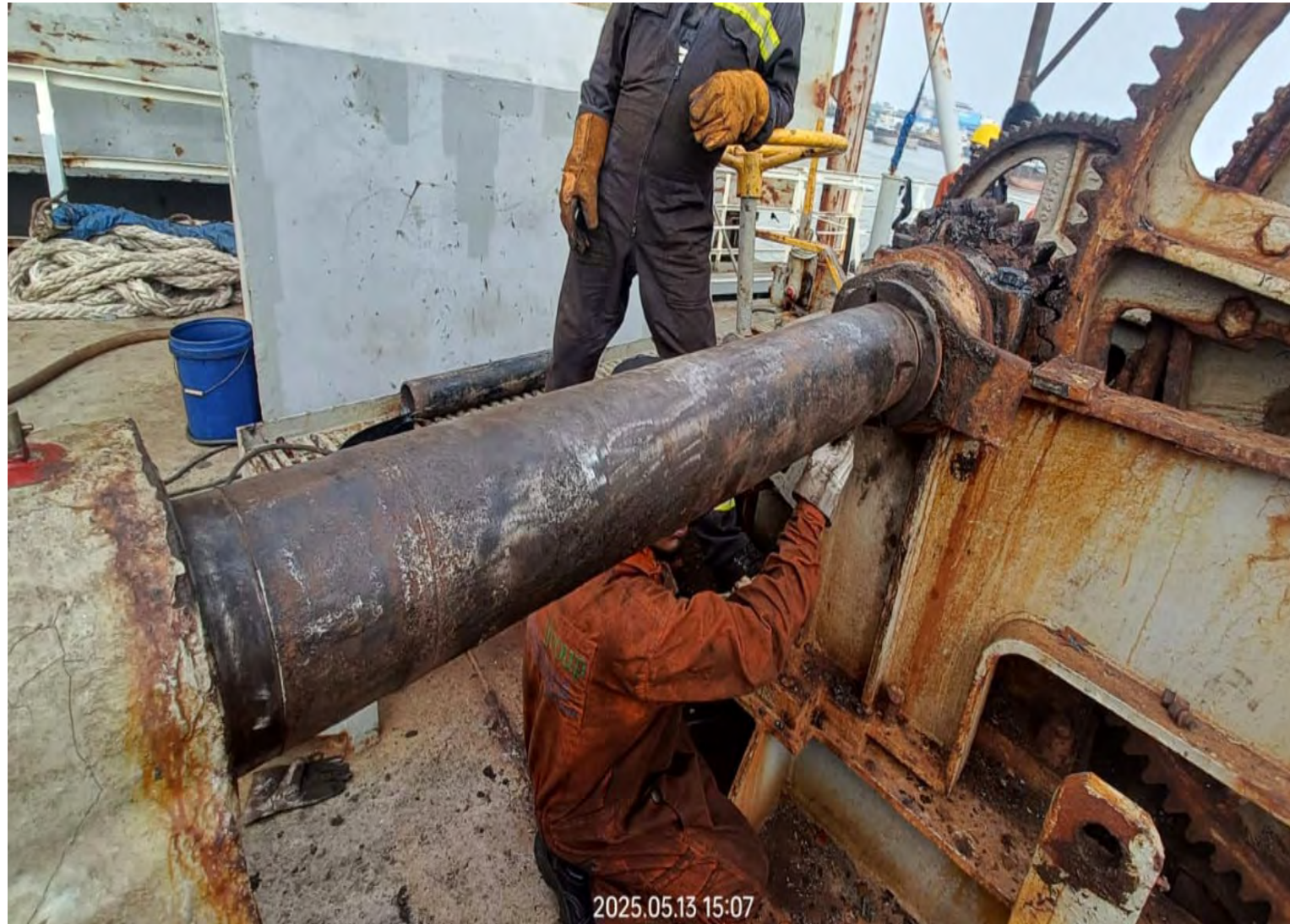
Effect of Clogged Grease Channel
