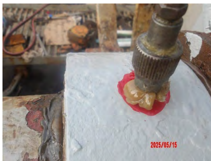
15 May- during greasing: Bush for side frame inner
