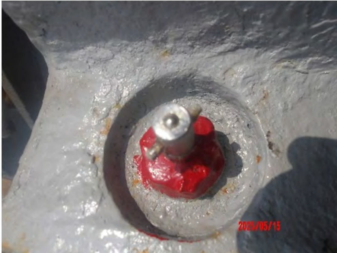
Before greasing of the Clutch for Hawser Drum Bush
