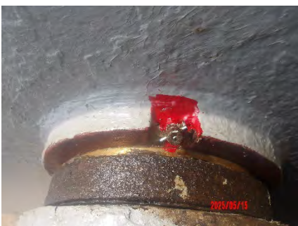
15 May- Before greasing: Bush for hawser drum outer point 1
