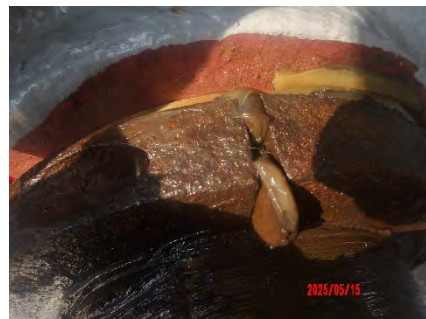
15 May- After greasing: Bush for hawser drum inner point 1
