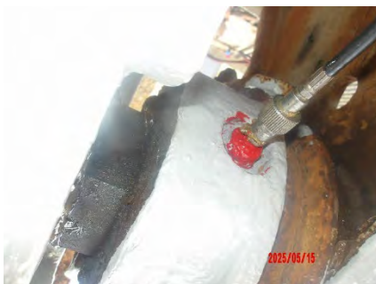
15 May- during greasing: Clutch of hawser drum 2
