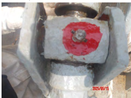
15 May – Before greasing: brake spindle greasing point
