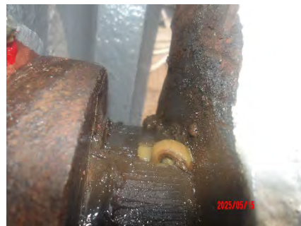
15 May- After greasing: Clutch of hawser drum 1
