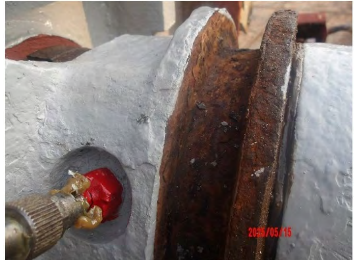
After greasing of the Clutch for Hawser drum bush
