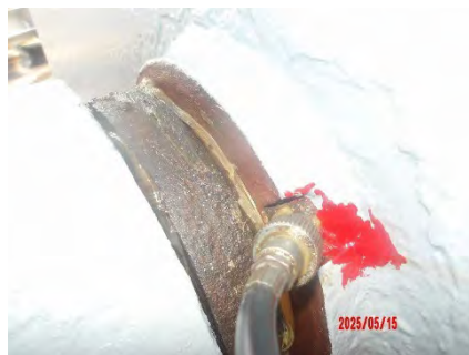
15 May- during greasing: Bush for hawser drum outer point 1
