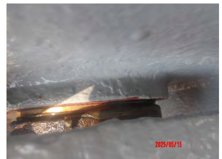
15 May- After greasing: Bush for hawser drum outer point 1
