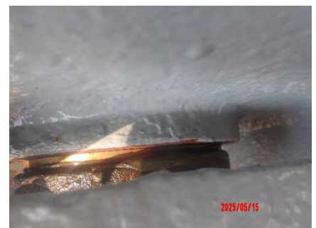
15 May- After greasing: Bush for hawser drum outer point 1
