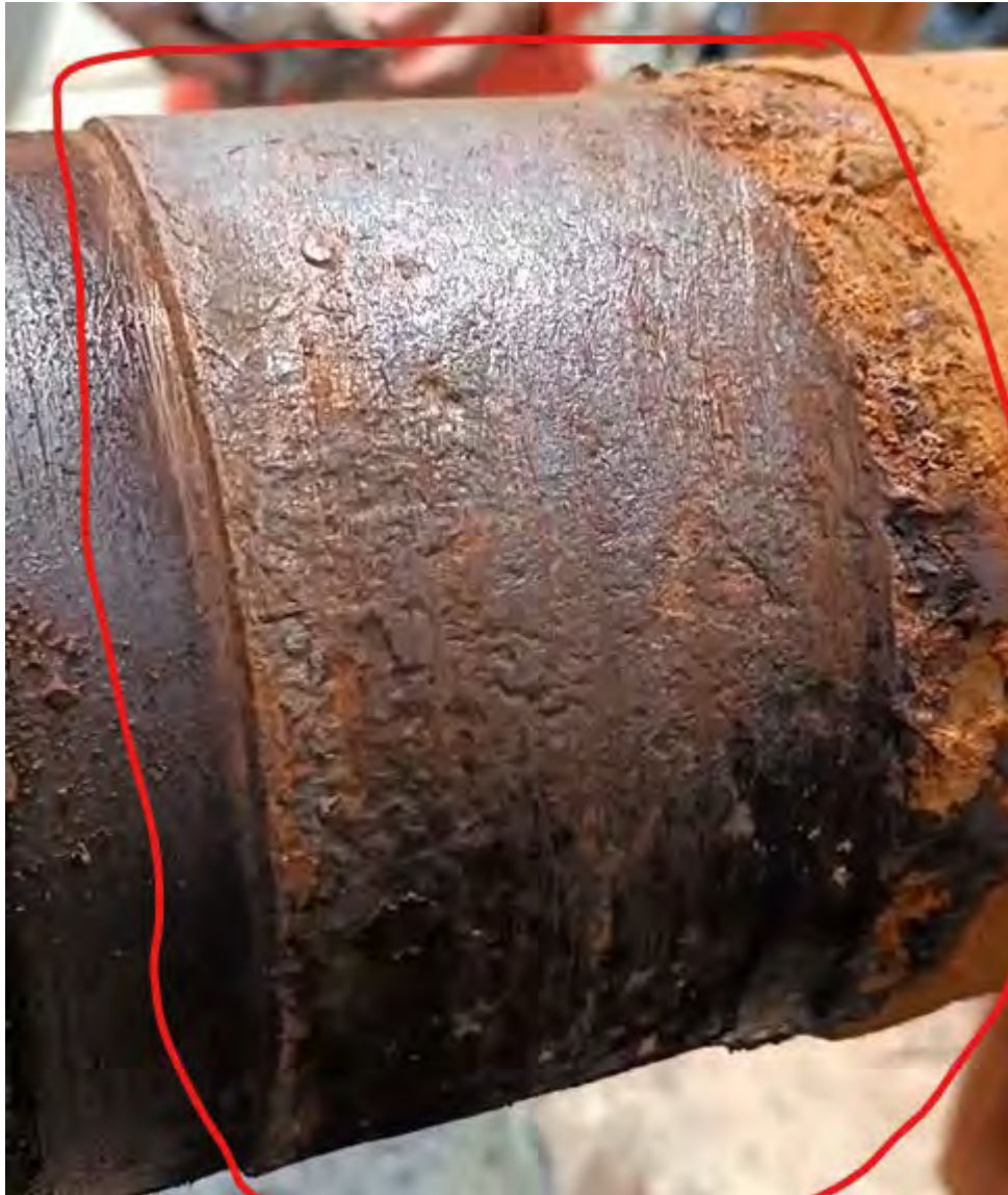
Effect of Clogged Grease Channel
