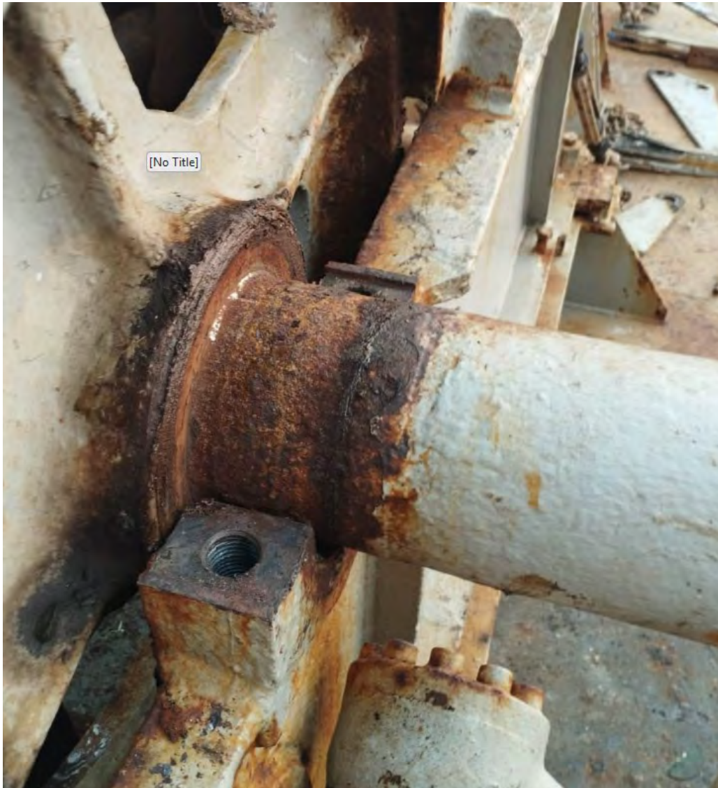
Effect of Clogged Grease Channel
