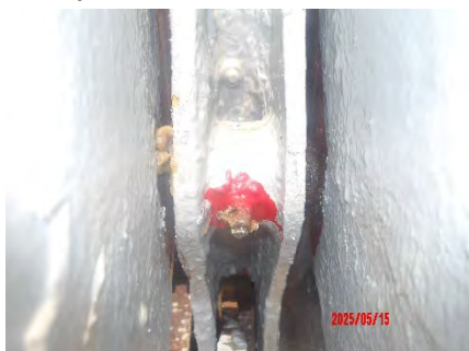
15 May – Before greasing: brake band joint 4
