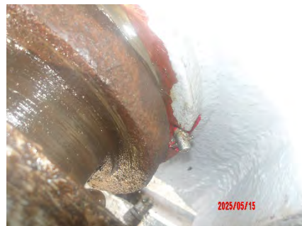
15 May- after greasing: Bush for hawser drum inner point 2
