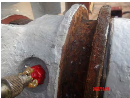
15 May- during greasing: Clutch of hawser drum 1
