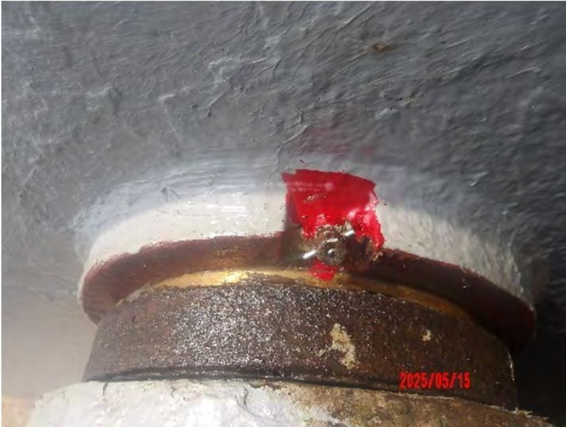
Before greasing of the Inner Hawser Drum Bush
