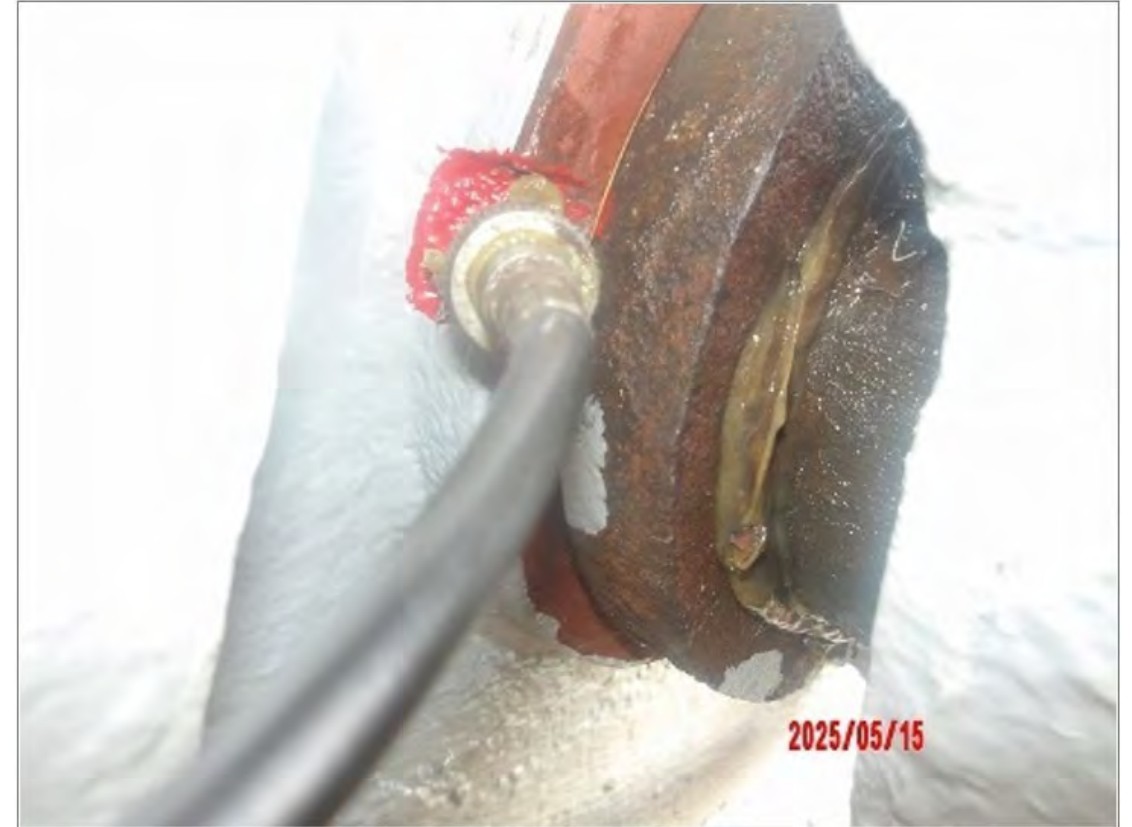
After greasing of the outer Hawser drum bush
