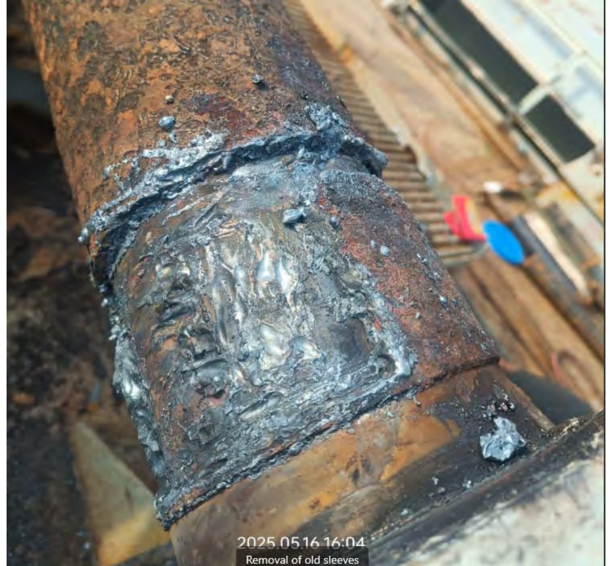
Effect of Clogged Grease Channel
