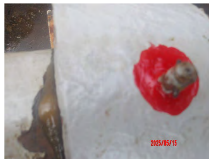
15 May- After greasing: Bush for side frame inner
