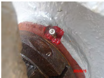
15 May- Before greasing: Bush for hawser drum inner point 2
