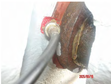
15 May- during greasing: Bush for hawser drum inner point 2
