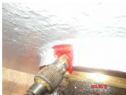
15 May- during greasing: Bush for hawser drum outer point 1
